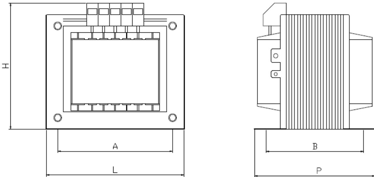
**Technical data:** Input 230-400.V at 50/60 Hz and Output 2x12.V, 2x24.V, 2x55.V, 2x115.V (2x12 and 2x24 since to 1600.VA)
